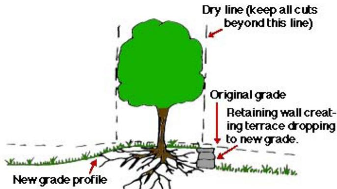
Fig 4. Grade around existing tree should be lowered as illustrated above. The choice between slope or wall will depend upon the space available and the appearance desired.
